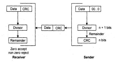
If the string arrives without error, the CRC checker yields a remainder of zero and the data unit passes. If the string has been changed in transit the division yields a non-zero remainder and the data unit does not pass.
